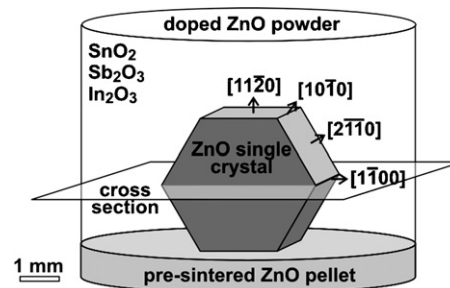
Fig. 1. Experimental set-up for sintering ZnO single crystals embedded in ZnO powder with the addition of three IB-forming dopants having different oxidation states: SnO 2 , Sb 2 O 3 and In 2 O 3 .
